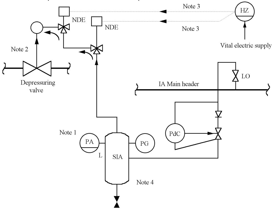
SIA = Secure Instrument Air
