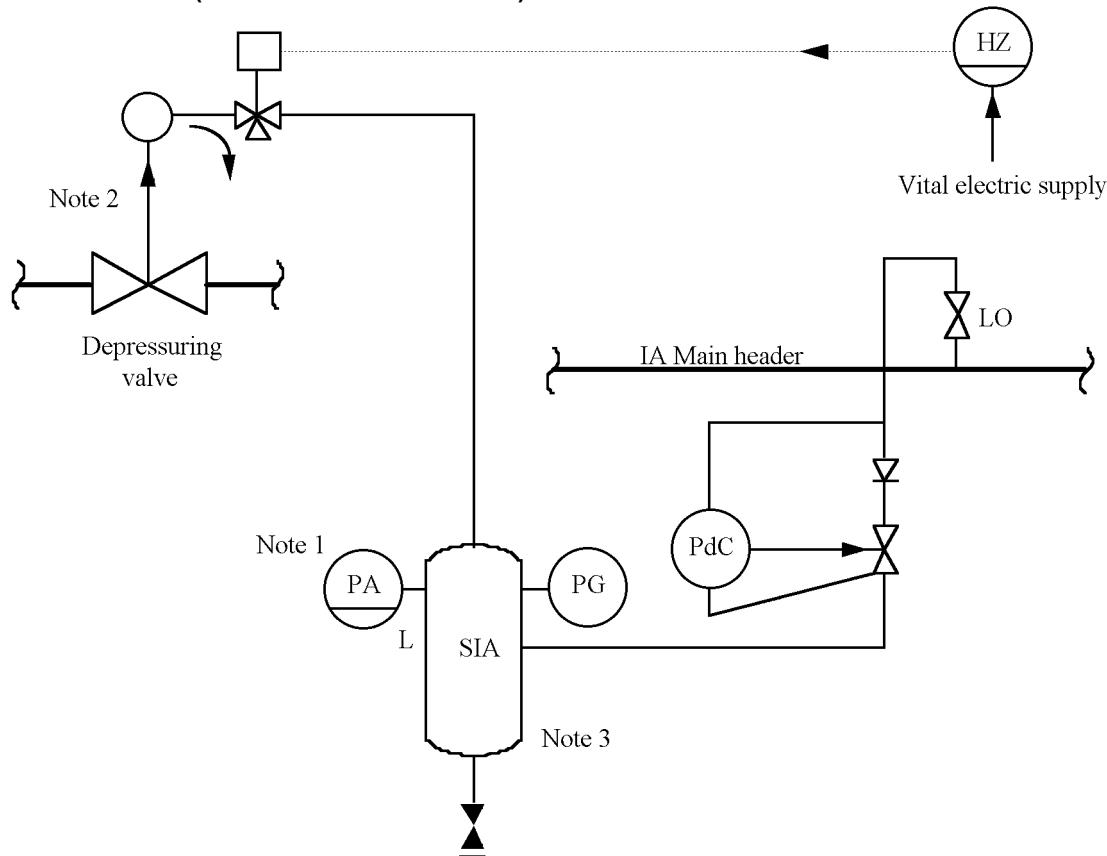
SIA = Secure Instrument Air
